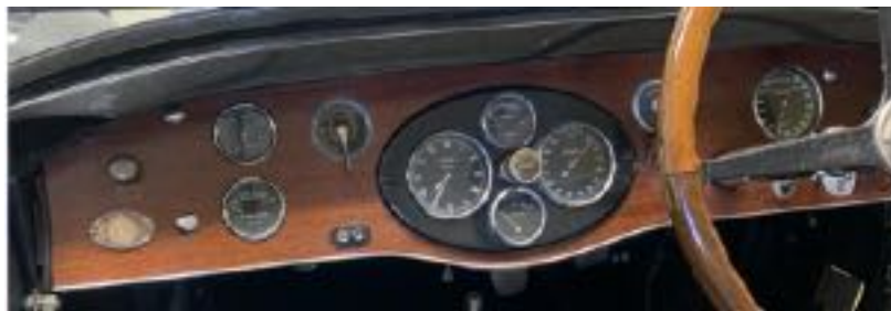
The standard dashboard of a type 40 had just four instruments in the middle: A revolution counter, an oil pressure gauge, and amperemeter and a clock in the centre section but no speedometer! Jacques Messian also wanted a speedometer (right), a Le Nivex fuel level gauge (a manometer) and an O.S. water temperature gauge (both on the left)
