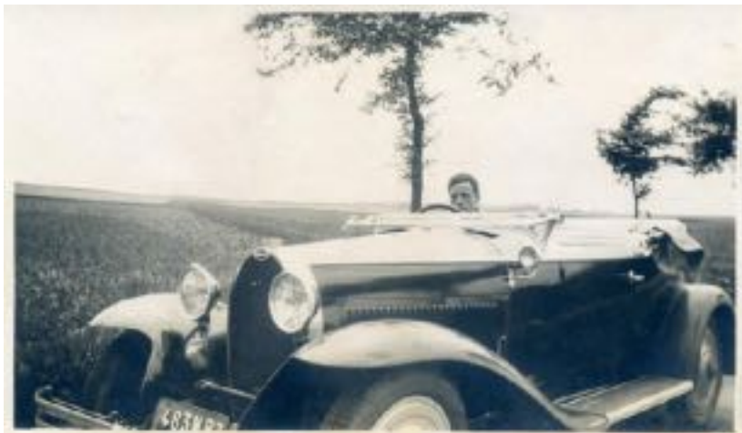
The young Jacques Messian when the car was new and with its first license plate. Note it has narrow double bumpers and wheel disks. Also note it did not have suicide opening doors and it also has separate cowl lamps on the side, like the prototype and the Chrysler 72 roadster but in this case, they were Marchal's (Photo Pierre Yves Laugier)
