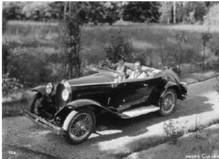
Promotional picture of the prototype Jean Bugatti roadster 40698. Note the large American style bumpers and the nickel or chrome plated wire wheels. Ettore was very much against chrome plating. He did not like it and compared it with doublé (gold plated copper or bronze). Promotional picture made by the official photographer of the factory, the firm Carabin in Strasbourg # 184.
