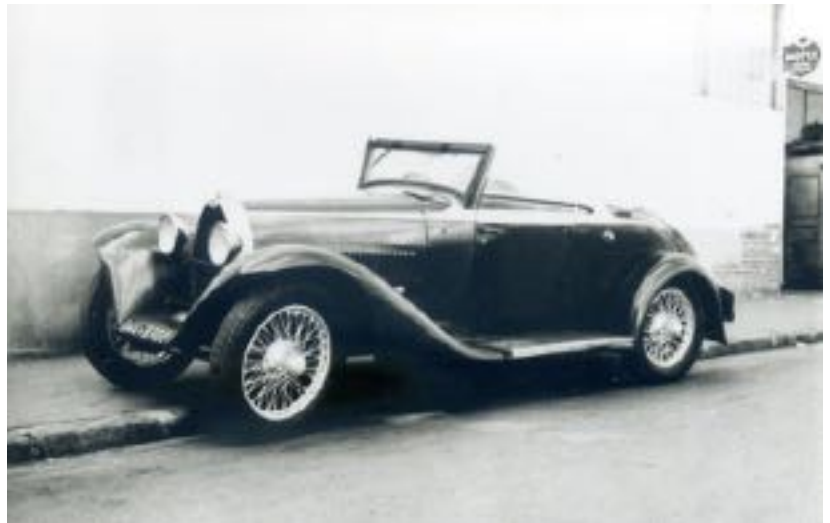
When in the ownership of Lartizien in Paris. The car had been 'modernized' by modifying the shape of the front fenders with a straight insert; changing the windscreen and the doors are now suicide doors. The wheel disks and the cowl lights have been removed. (Photo Pierre Yves Laugier).
