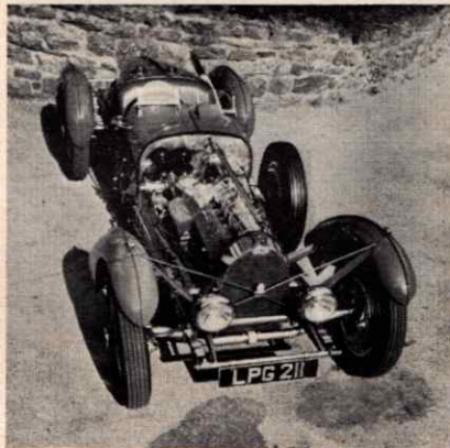
Mudguards and lights were added to Grand Prix car by English owner. Note Bugatti's "split" front axle.
